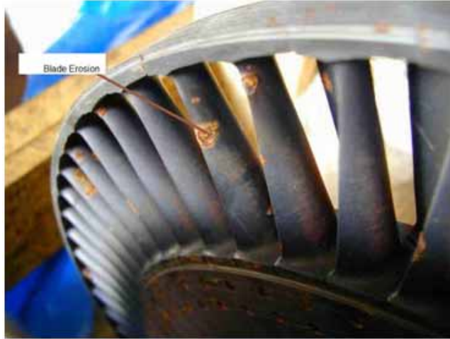
Figure 2. Water impingement on turbine blades
