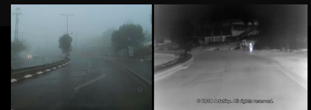
Wxga CMOS dashcam AdaSky's VIPER FIR solution
