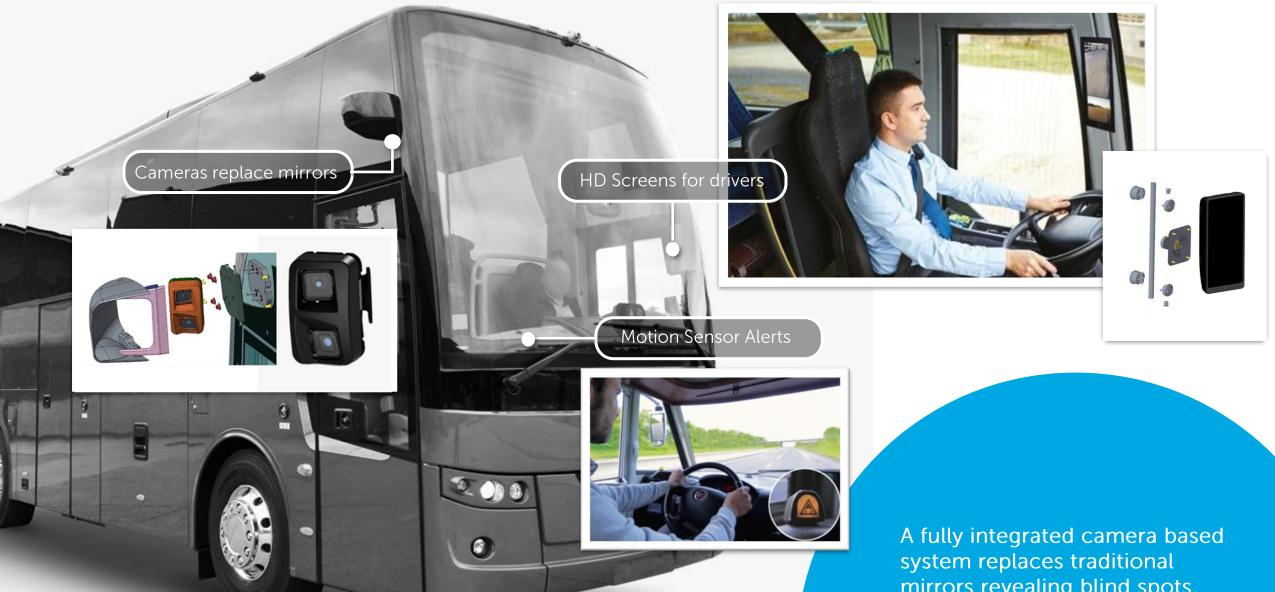
A fully integrated camera based system replaces traditional mirrors revealing blind spots through real time image analysis and notifications for reduced accidents and safer driving
